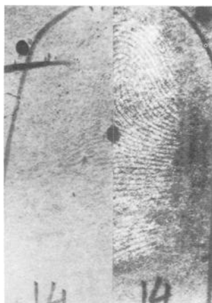
FIG. 10—Fingerprint on yellow envelope paper developed with ninhydrin and enhanced with zinc nitrate on the left and cadmium nitrate on the right. Photograph taken under optimal excitation/emission conditions for zinc complex photoluminescence and under optimal conditions for cadmium complex photoluminescence, respectively.
