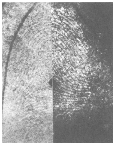
FIG. 2—Weak fingerprint developed by overheating the ninhydrin reaction. Left: enhanced with zinc nitrate. Right: enhanced with cadmium nitrate. (Photographic conditions ideal for zinc-RP and cadmium-RP complexes, respectively.)
